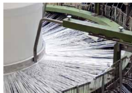
TUBETEX™ continuous production on a tubular loom
