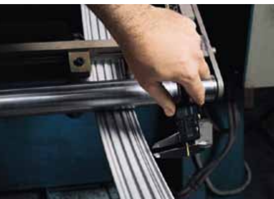
Quality control during the profile extrusion process
